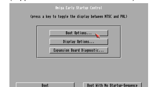
The Early Startup screen makes fault finding easier, as long as your graphics set-up can display it!
